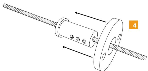
**7** Pull all parts together and mount into the wall with the screws.
