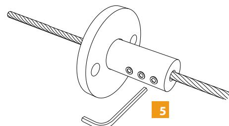
**3** Feed cable through 1.5" round cylinder for holding cable.
