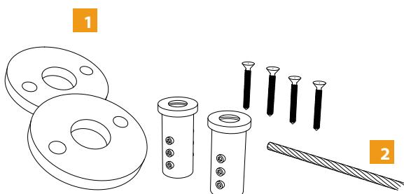
**5** Tighten down set screws on 1.5" round cylinder so the cable is secured.
